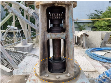
Example of good practice with oil leak prevention in the lower section of the mixer motor
